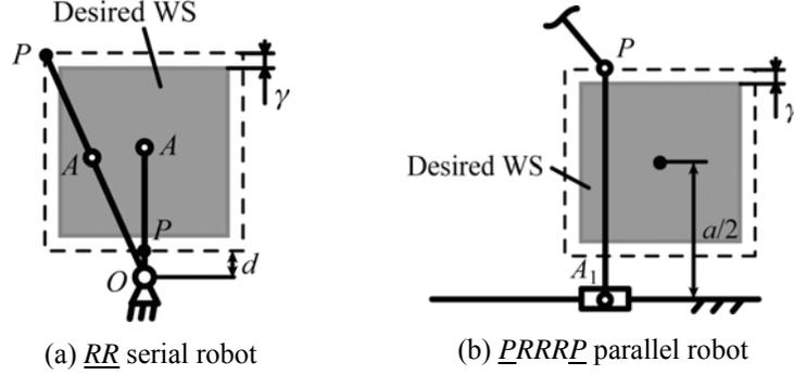
Fig. 2. Design constraints for obtaining the desired workspace.
