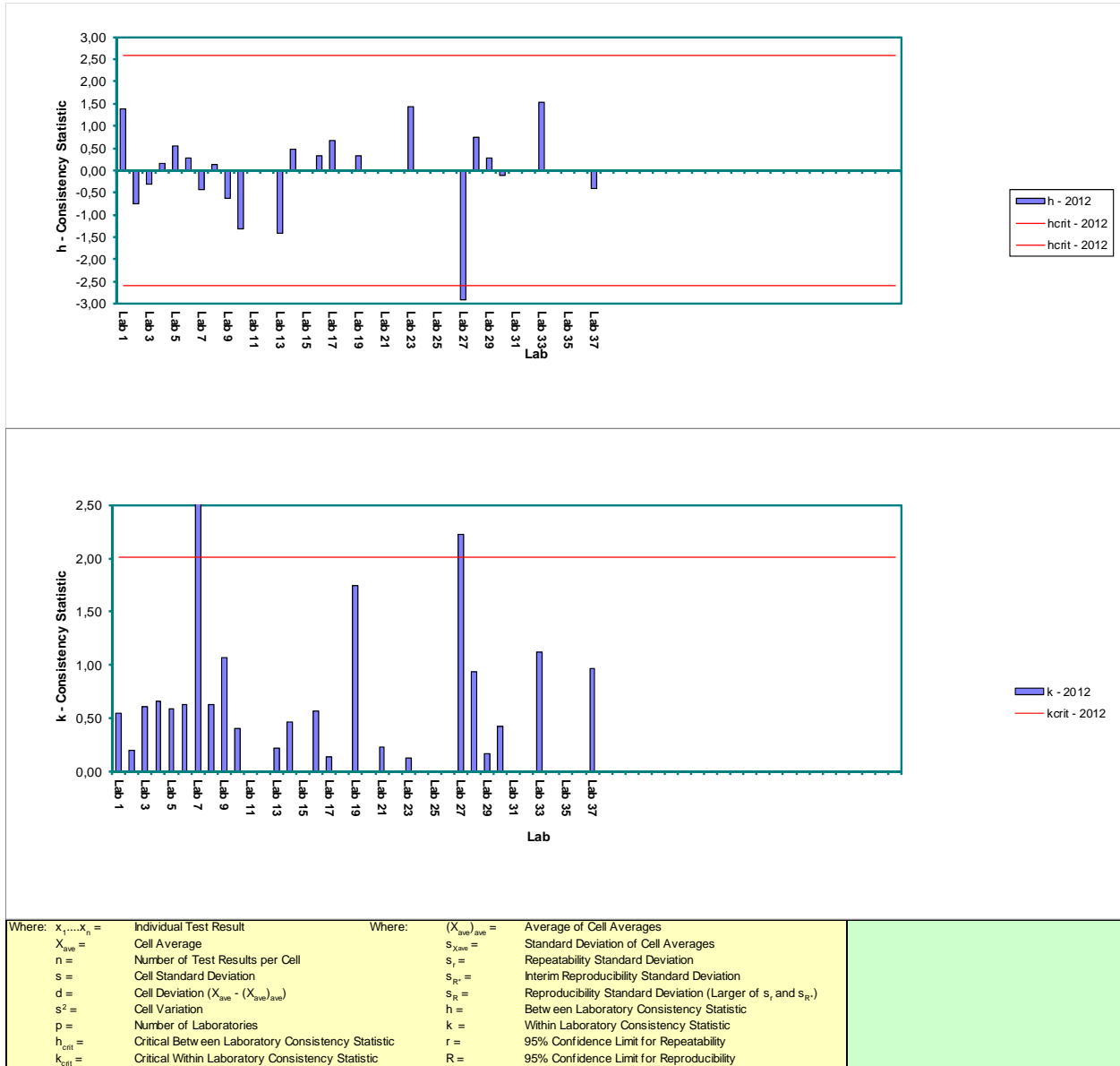
Figure 9.2 Voids Filled with Asphalt Mechanical Compaction
