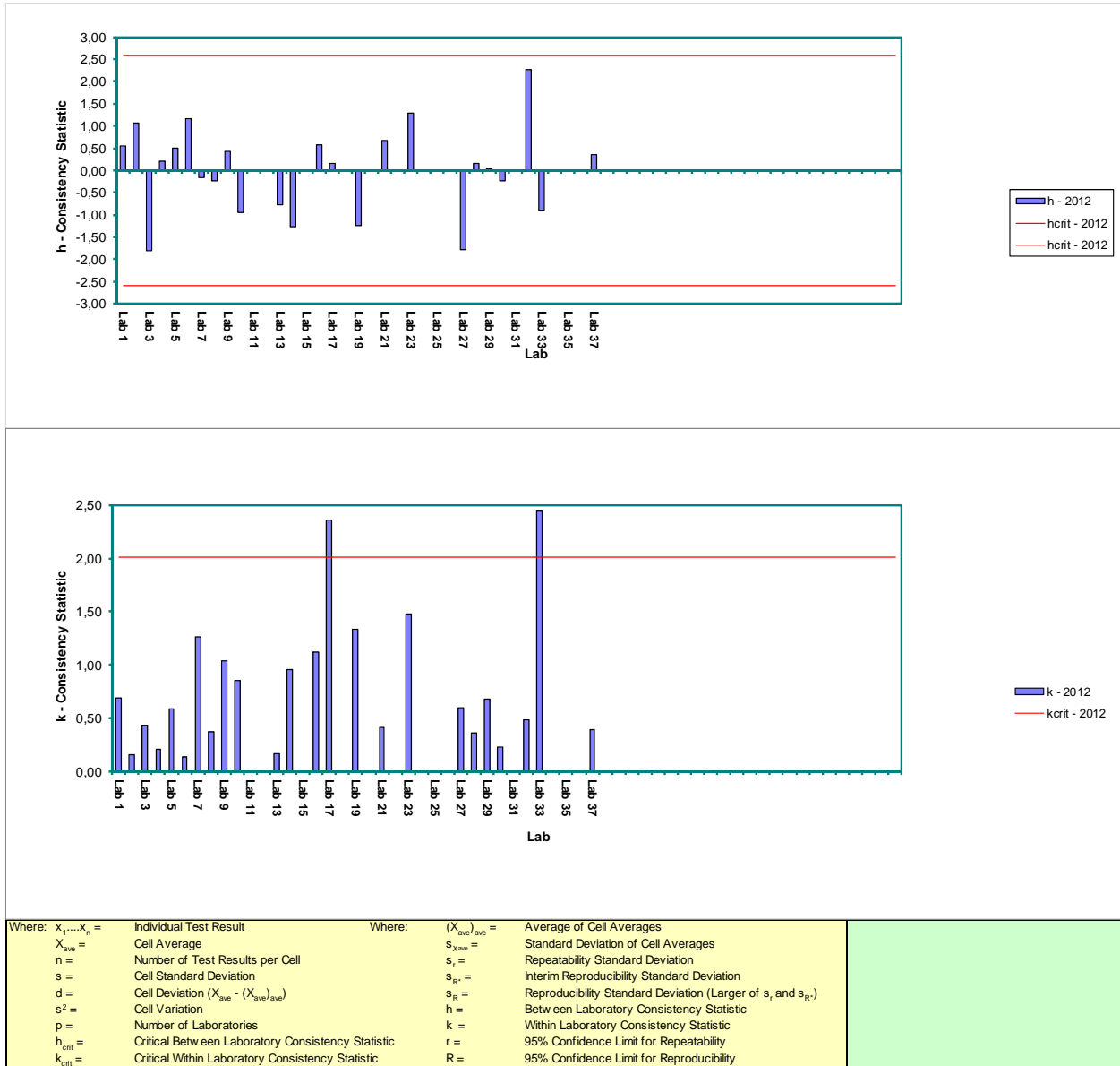
Figure 5.2 Marshall Stability Mechanical Compaction
