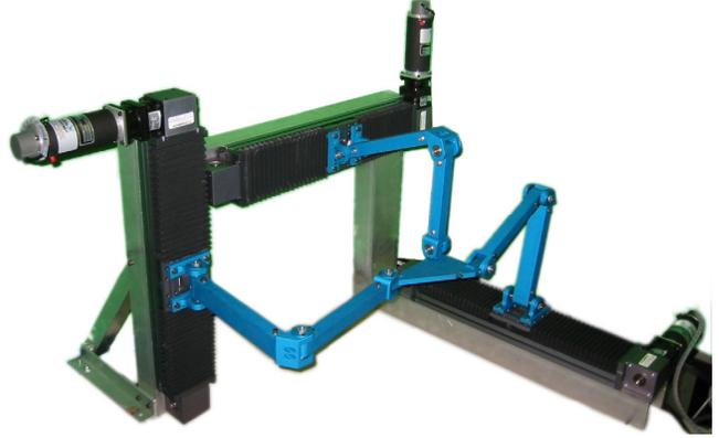
Figure 1. The Tripteron Cartesian parallel robot [2].
