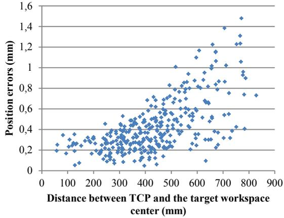
Figure 9. Position errors after calibration in the constrained workspace.
