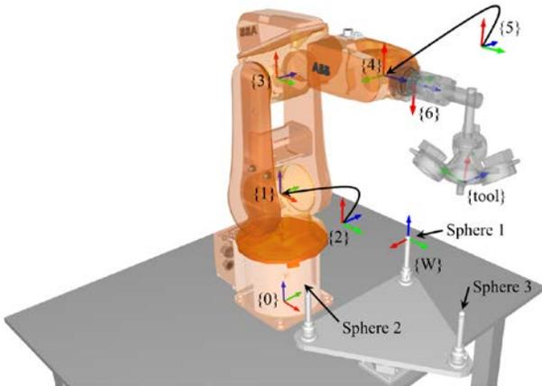
Figure 1. Reference frames of the IRB 120 robot.
