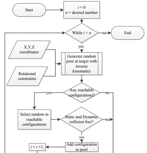
Figure 6. Algorithm for generating random robot configurations, free of static and dynamic collisions.
