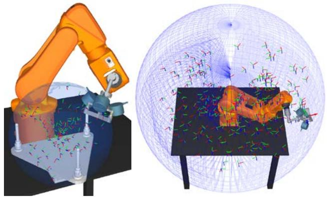
Figure 7. Random tool poses generated for measurements within the target workspace (left) and the whole robot workspace (right).
