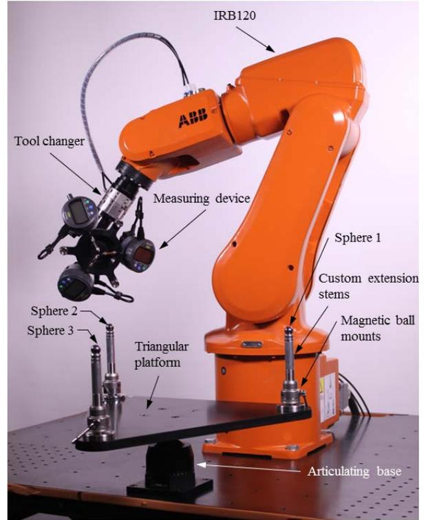
Figure 2. *TriCal*'s measuring device, installed on the IRB 120 robot, with the triangular platform installed on the table.
