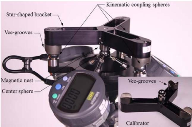
Figure 4. The *TriCal*'s measuring device and its calibrator.
