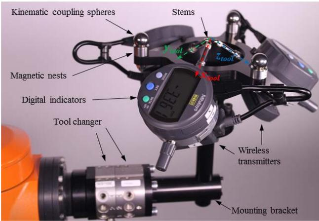
Figure 3. Components of the *TriCal*'s measuring device.
