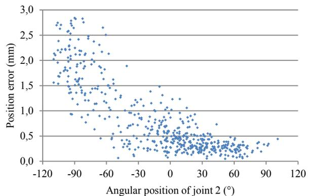
Figure 8. Position errors w.r.t. the angular position of joint 2 on the 500 configurations used for validation in the whole workspace.
