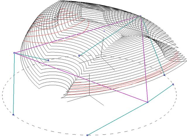
**Fig. 10 Constant-orientation workspace and singularity loci for a Rotobot design.**
