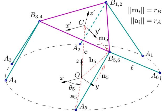
Fig. 2 Schematic and notation of the Rotobot
