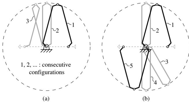
**Fig. 8 Passing through a self-intersection point by (a) changing or (b) keeping the branch index.**
