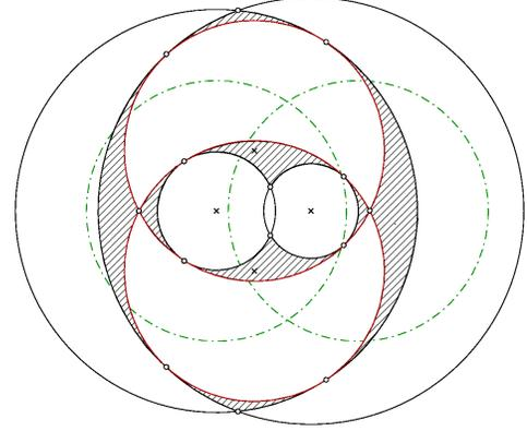
**Fig. 7 Horizontal cross-sections of a Bohemian dome and the corresponding vertex spaces**
