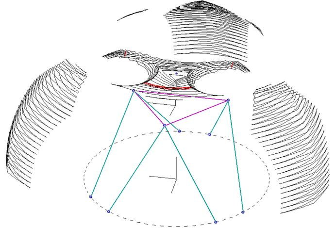
**Fig. 11 Constant-orientation workspace and singularity loci for a Rotobot design.**
