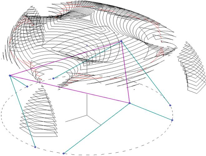
**Fig. 12 Constant-orientation workspace and singularity loci for a Rotobot design.**
