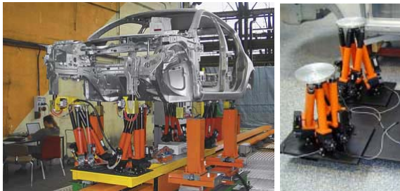
FIGURE 7 – FLEXPLP, UN SUPPORT RECONFIGURABLE (ABB)
