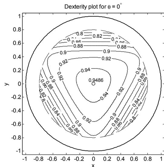
Fig. 5. Local dexterity contour plot for the parallel robot under study.
