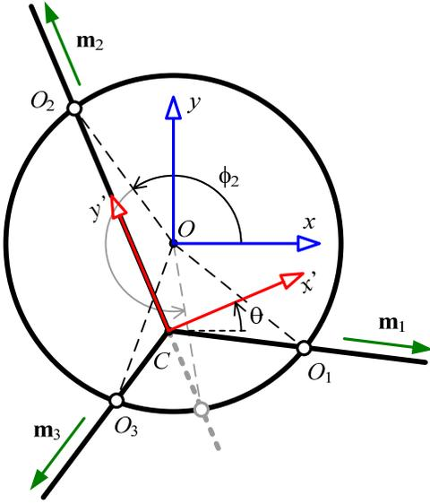
Fig. 2. Schematic of the parallel robot under study.
