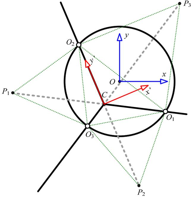
Fig. 3. Solving the direct kinematics of the parallel robot under study.
