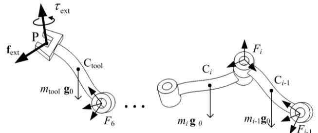
Figure 3. Schematics of the serial robot links under external load and the gravity effect
