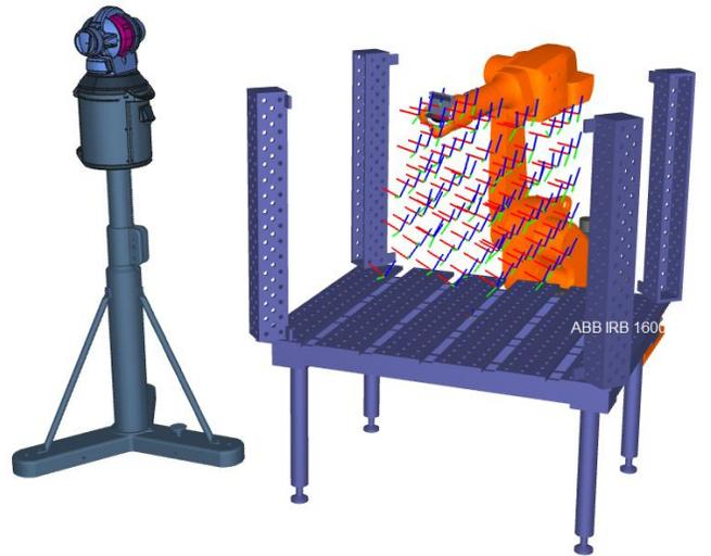
Figure 4. The 125 poses of the ABB robot end-effector which are generated inside the workspace of the cable-driven robot
