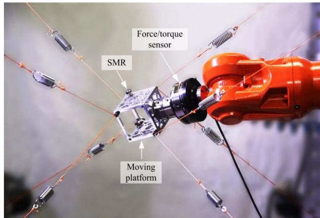
Figure 5. Connection of the moving platform of the cable-driven robot to the flange of the ABB robot
