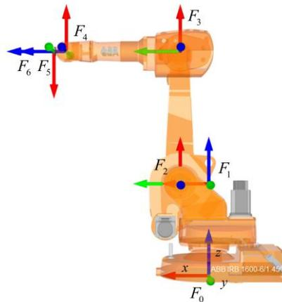
Figure 2. Frame assignment for the serial robot
