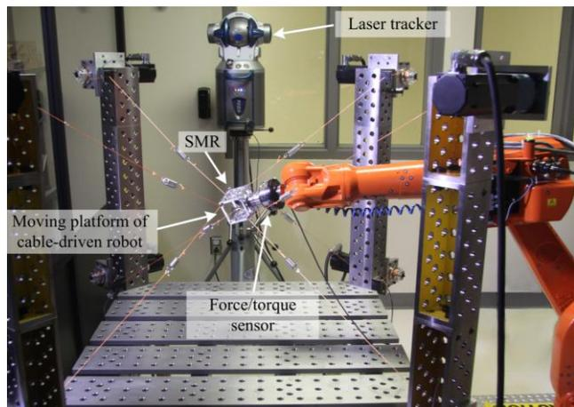
Figure 1. Experimental setup for elasto-geometrical calibration process of the ABB IRB 1600-6/1.45 robot
