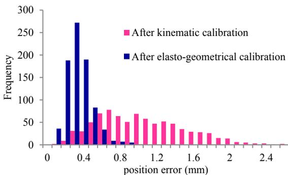
Figure 7. Histogram of the ABB robot position errors after kinematic calibration and after the proposed elasto-geometrical calibration
