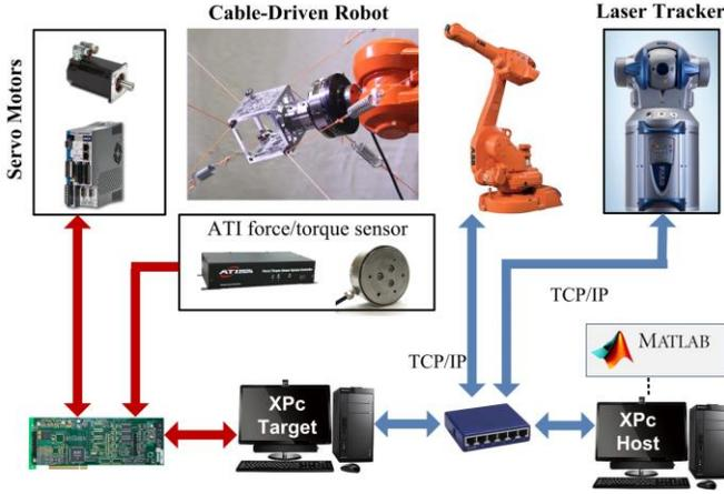
Figure 6. Hardware setup for control and measurement during the calibration process
