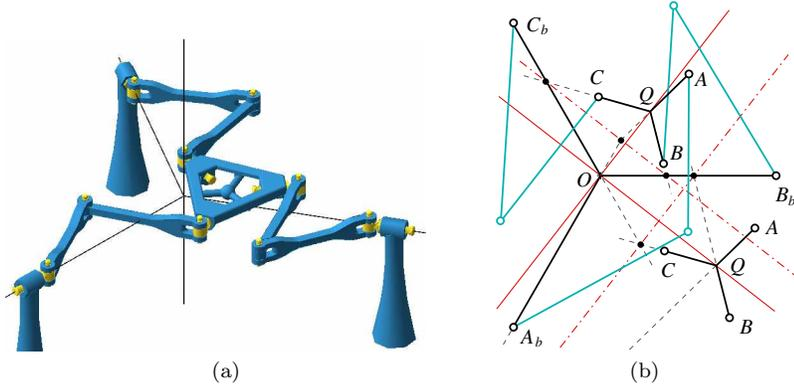
Figure 3. The planar mode: (a) face up; (b)  $\mathcal{C}$ -singularities face down.
