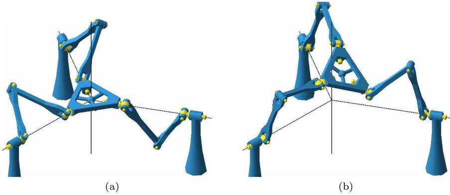
Figure 4. The DYMO chain in (a) lockup mode and (b) mixed mode.
