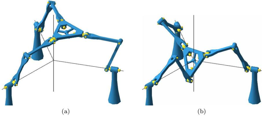
Figure 2. The DYMO chain in (a) translation mode and (b) orientation mode.
