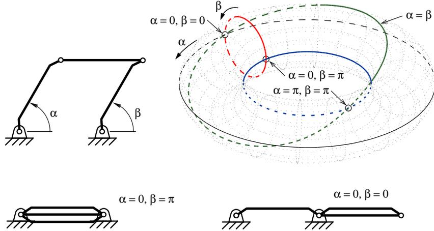
Figure 1. The equal-length four-bar mechanism, the  $\mathcal{C}$ -space and its singularities.
