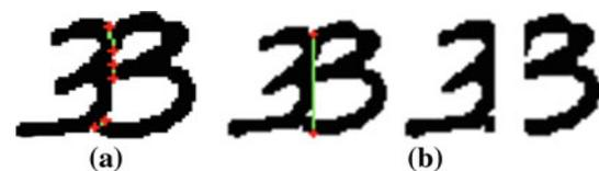
**Fig. 8** Segmentation points: **a** ground truth with six segmentation points and three segmentation paths and **b** segmentation path created by a segmentation algorithm and both segmented digits
